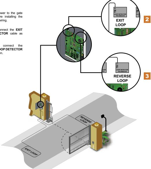
To protect the gated area from accidentally closing on vehicles a series of Loop Detectors must be installed. Loops are laid underneath, cut into asphalt or concrete driveways or buried beneath gravel and earth driveways. A Loop Detection system will sense a vehicle like a metal detector and send a signal to the gate operator preventing the gate from automatically closing on a vehicle when exiting.
