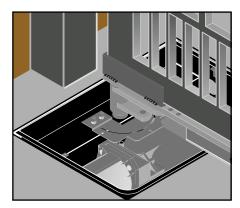
Install the gate on to the hinge and the U-Channel, gate should swing freely 90 degrees.
