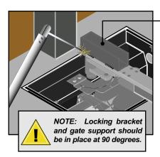
Weld the gate U-Channel onto the gate support bracket.
