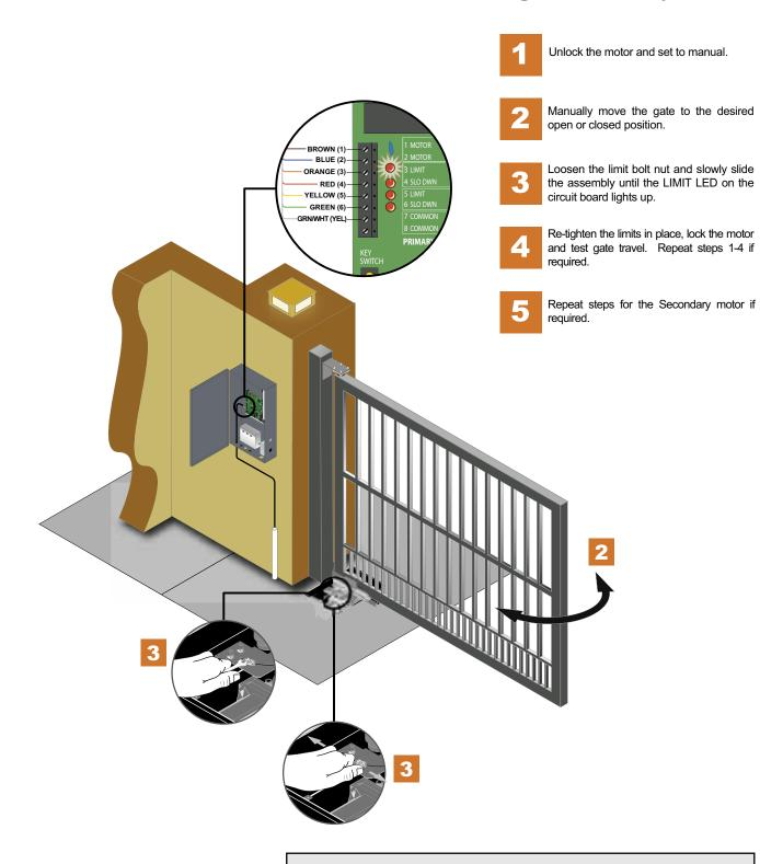
The limit switches on the motor can be adjusted to control the travel of the gate and to precisely set the full open and full closed position of the gate. This feature is especially useful in applications where the gate opens partially, such as on a curved driveway.
