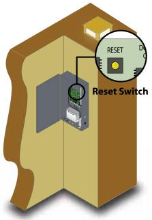
When the operator is in hard shutdown condition (audio alarm "chirps" every 5 seconds), the only way to reset the gate operator and return it to normal operation is to activate the reset button located on the top of the PC Board (**see illustration above**), pressing this button will reset the gate operator to normal operation, but will not activate the gate operator. An external alarm-reset switch can be mounted provided it is installed in the line of sight of the gate and gate operator.
