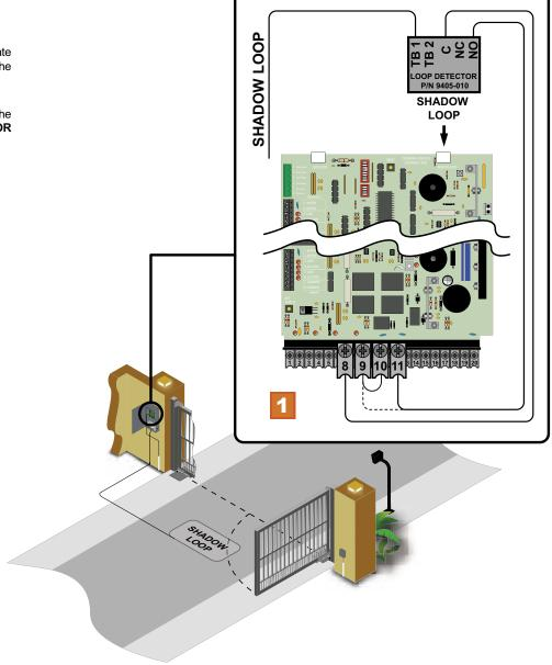
A Shadow Loop is placed inside the swing gate area to prevent the gate from closing on a vehicle that is in the path of the gate after the open time has expired or the Exit Loop is too far back from the Reverse Loop. The Shadow Loop is only active when the gate is in the full open position and will not allow the swing gate to close. Once the close cycle begins the Shadow loop will not reverse the gate.
