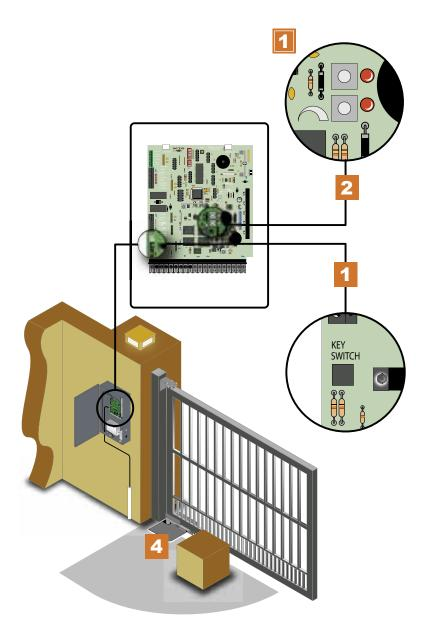
This vehicular gate operator is equipped with an inherent adjustable reverse sensor (Type A) that is used as the primary entrapment sensing system. When sensing an obstruction in either the opening or closing gate cycle, the gate operator will reverse direction. For this system to function correctly, the gate must be properly installed and work freely in both directions. A good set of roller bearing hinges are essential for proper swing gate operation.
