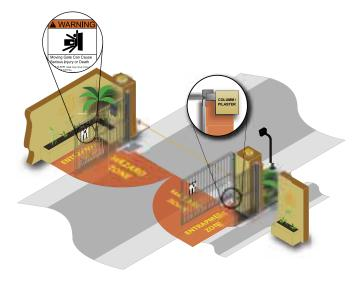
This vehicular gate operator is equipped with an inherent adjustable current sensing system (Type A). This system will sense an obstruction in both the opening and closing cycles causing the gate to reverse direction should an obstruction be encountered. If the system detects a second obstruction before reaching the full open or close limit after the initial reversal, an alarm will activate and the operator will need to be reset before resuming normal operation (see pages 21-23).
