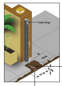
Remove components from the foundation box before setting in to place.
